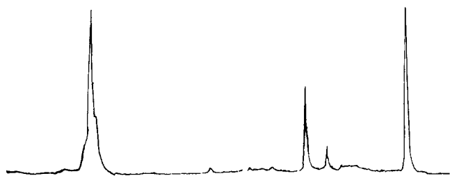
Fig. 3.—N.m.r. spectrum for a mixture of cis - and trans -3,5-diphenyl-2-methyl-2-penten-4-ynoic acids (IIIE, R = H). The maxima are, from left to right, at 2.27 (low), 2.75 (Ar-H), three unassigned minor peaks, 7.51 (C-2 CH 3 , cis ), 8.17 τ (C-2 CH 3 , trans ), a broad unassigned minor peak, and tetramethylsilane.
